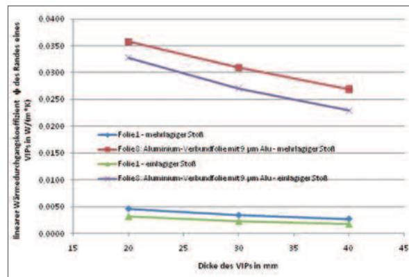
Linear thermal transmittance of high-barrier and ultra-barrier films
