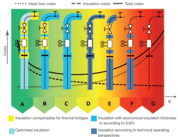
Figure 3: Energy efficiency classes of insulation based on longitudinal heat loss flow
