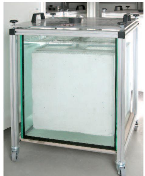
Water absorption of EPS with high thickness
